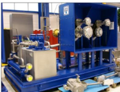
control instruments and speed converter with 4-20 mA output signals, complete lube oil system consisting of reservoir, lube oil pump, standard lube oil cooler, dual oil filter.
